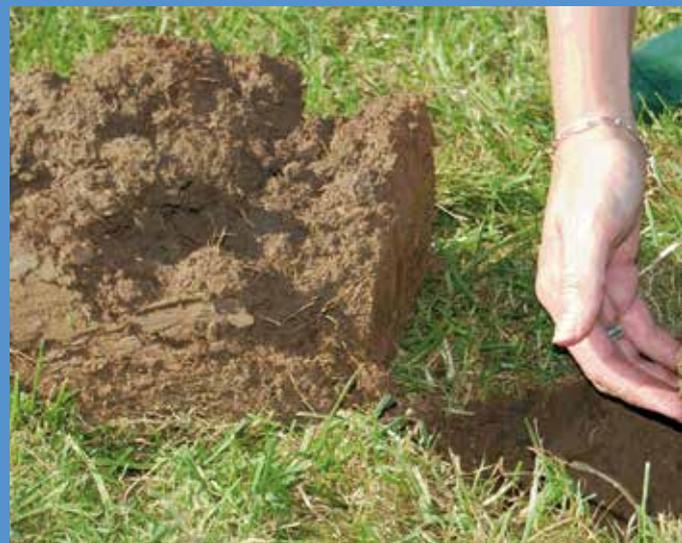
30cm, by cutting down three sides and then levering the block out to observe the undisturbed side of the soil. Gently break up the block, to assess for compaction:
